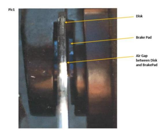
Pic 1 shows an out of adjustment brake caliper. The pic was taken looking down from the top of the front wheel. Notice the **Air Gap** to the right, but no **Air Gap** exists on the left.
