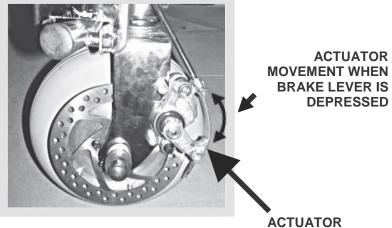
If the actuator is not fully engaged, (additional movement <u>is</u> possible by moving the actuator by hand when the brake lever is fully depressed) and the hand movement of the actuator causes the front wheel to become locked, then see Disc Brake Level Adjustment section below. The brake pressure adjustment should not be necessary because the cable has slipped or stretched over time. If this is not the case, then adjust the braking pressure.
