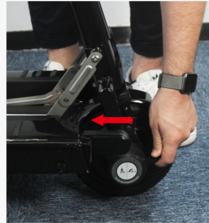
Figure 21. Securing the Freewheel
