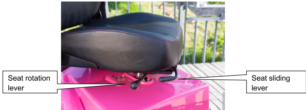
Figure 14: Seat rotation and front-to-back adjustment levers
