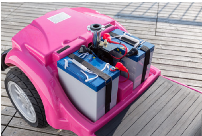
Figure 7: Batteries and battery connections
