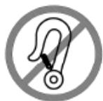
Figure 7 – Symbol for information not intended to be used as a seat in a motor vehicle
