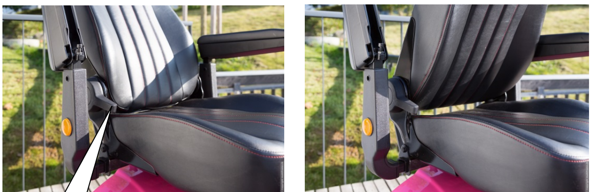
Figure 13: Seat backrest adjustment lever
