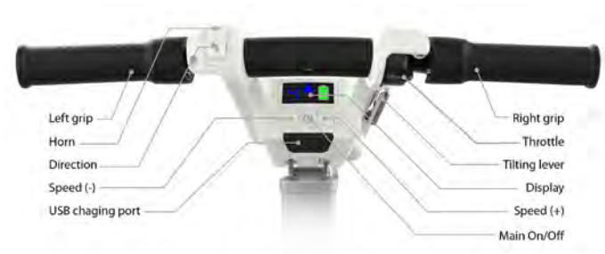
Figure 27 Driving Console overview
