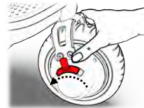
Figure 59 Securing the freewheel
