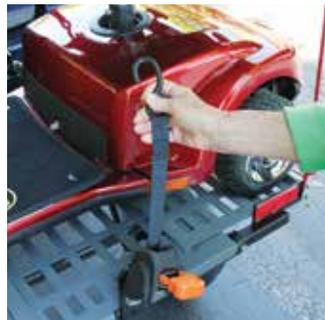
Self-tensioning retractable securement belts.
